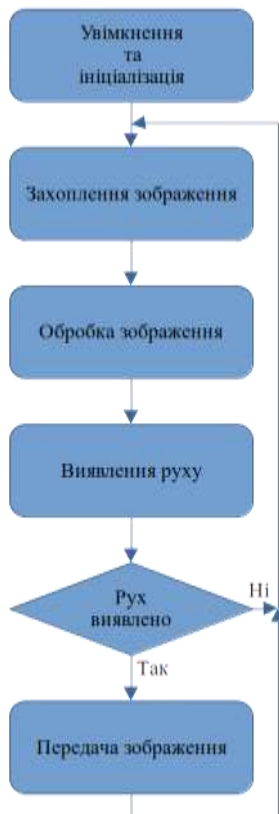
Рис.3. Циклограма роботи модуля DFRobot FireBeetle 2 Board ESP32-S3 N16R8 with Camera
