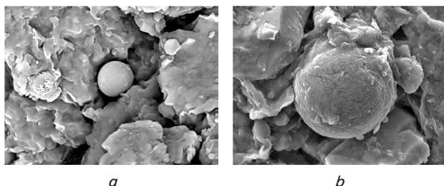
Fig. 2. Microinclusions in the highly dispersed fraction of bentonites: *a* – spherical particles of allophane in montmorillonite; *b* – titanium-containing particles in montmorillonite
