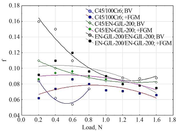
Fig. 6. Dependence of the coefficient of friction on the load when testing pairs of steel 45/ShKh15, steel 45/SCh 200 and SCh 200/SCh 200 in the basic version and with the addition of friction geomodifiers
