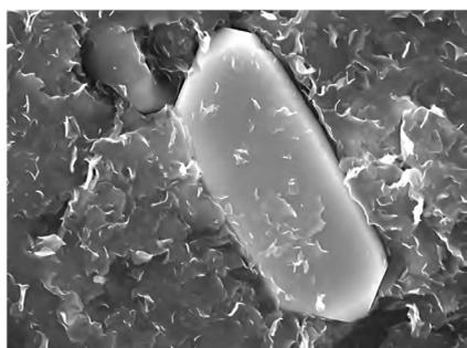
Fig. 1. Barite crystal in bentonite clay (Area of the image viewer field – 1000 μm<sup>2</sup>)
