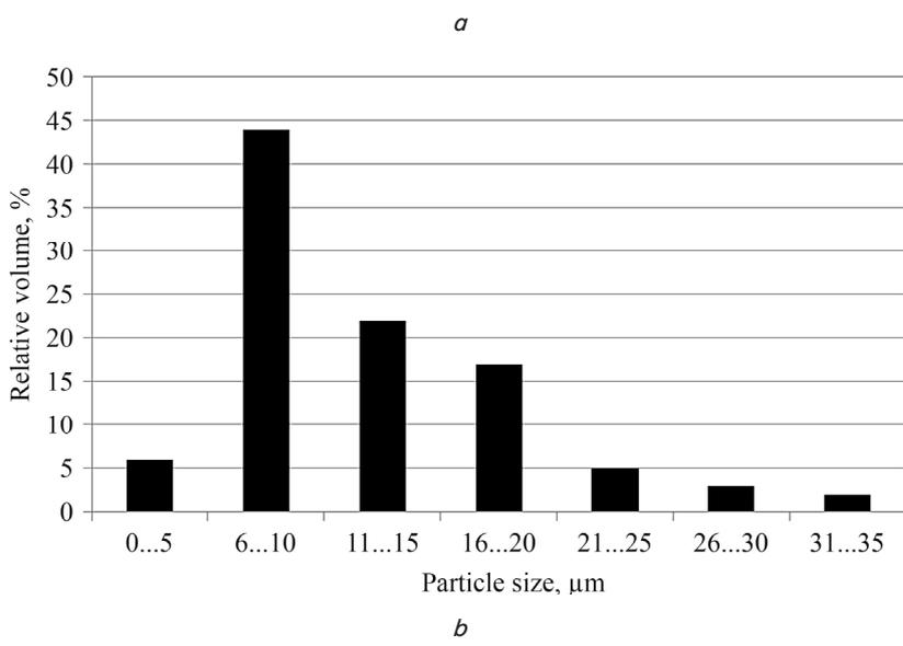
Fig. 3. Determining the size of particles of the serpentine powder: *a* – photograph of the microstructure 400×; *b* – particle size distribution histogram
