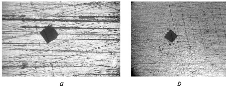
Fig. 8. Microphotograph of the surface of the sample with a measuring hole: *a* – basic version; *b* – variant with the addition of friction geomodifiers,  $\times 400$
