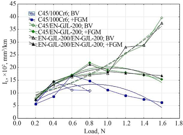
Fig. 5. Plots of wear intensity for pairs “steel 45/ShKh15”, “steel 45/SCh 200” and “SCh 200/SCh 200” in the basic version and with the addition of friction geomodifiers
