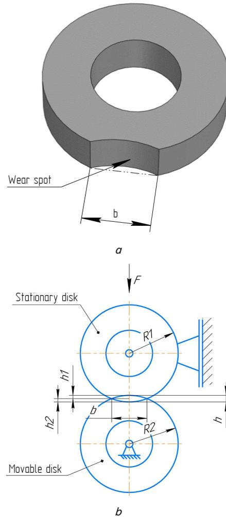
Fig. 4. Scheme for determining the volume of worn material: a – the location of the hole on the cylindrical surface of the stationary disk; b – scheme for calculating the wear depth
