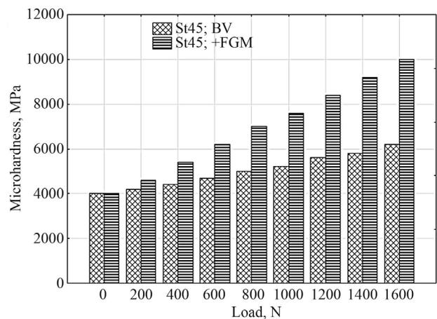
Fig. 7. Transformation of microhardness of tribosurfaces from load
