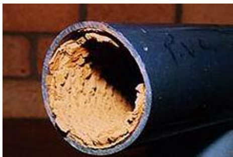
Fig. 4.12. Limescale in a PVC pipe. Fig. 4.13. Ion exchange resin in the form of beads.
