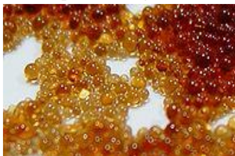
Fig. 4.12. Limescale in a PVC pipe. Fig. 4.13. Ion exchange resin in the form of beads.
