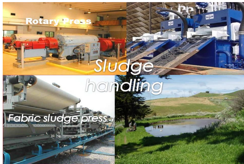
Fig. 4.30. Sewage sludge dewatering.
