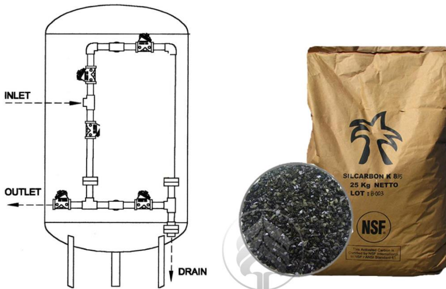
Fig. 4.27. Principal sketch of pressure filter (left) which may be filled with activated carbon (right).
