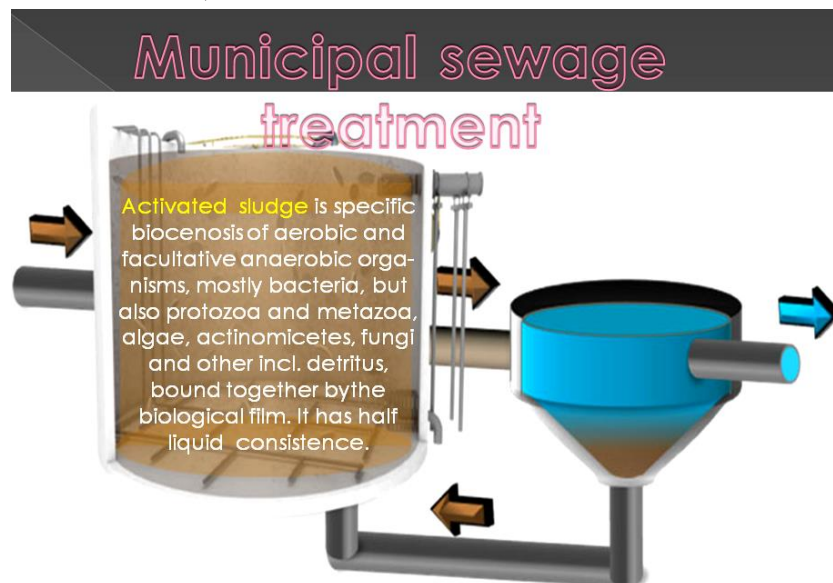
Fig. 4.19. Sketch of secondary sewage treatment in activated sludge tank connected with secondary clarifier (activation – intensification of processes ongoing in nature).
