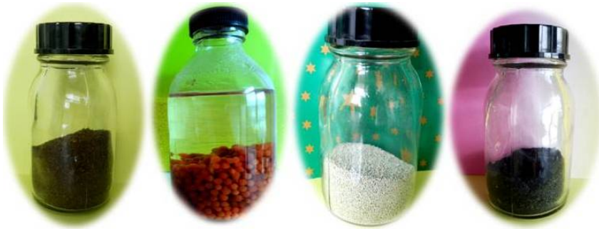
Fig. 1. Illustration of zeolite based adsorbents synthesized at laboratory. FeO(OH)-MnOx-zeolite, Fe(III)alginate zeolitic beads, ODA-zeolite and carbonized zeolite (from the left to the right).
