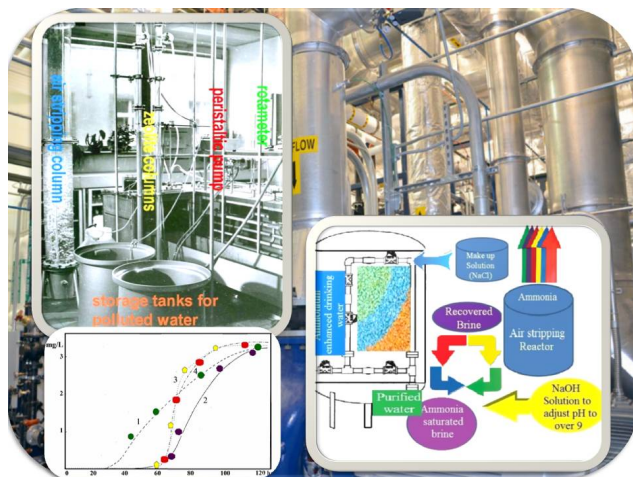
Fig. 6. Laboratory pilot for ammonium removal out of the simulated drinking water (upper left photograph) and typical breakthrough curves during the process studied (left down). Principal sketch of zeolite ion exchange pilot installation (ZIEPI) situated at the field experimental facility of Water Research Institute (right down).
