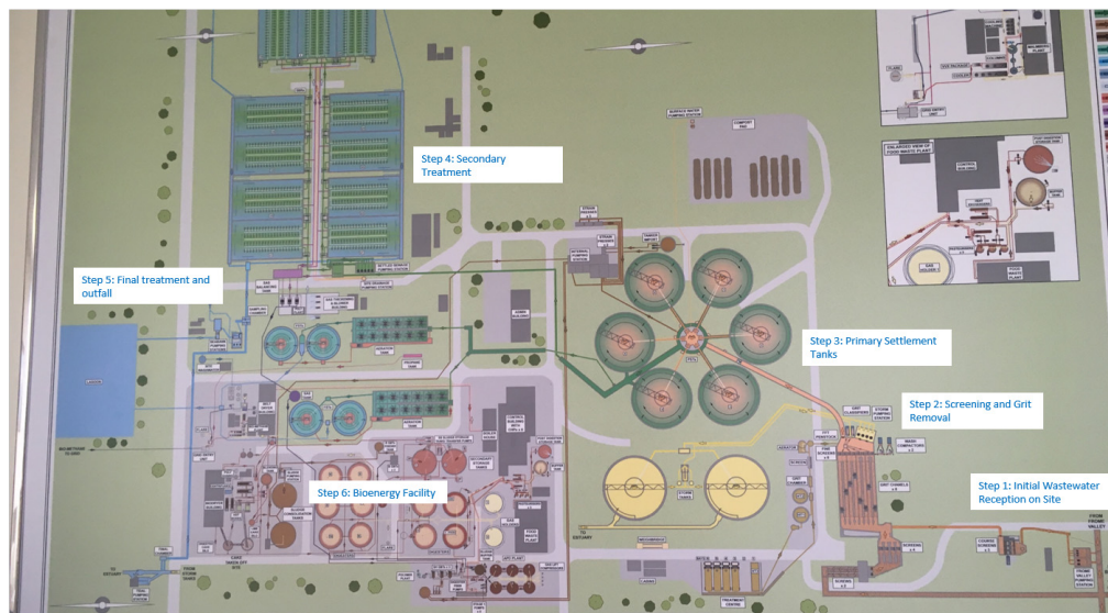
Fig. 1. Schematic of Avonmouth WwTW, including the Bioenergy facility (Source: Wessex Water)
