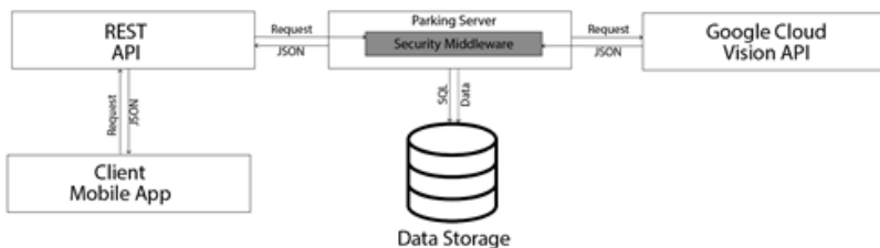
Figure 2 - Smart Parking Software Architecture using Security Middleware
